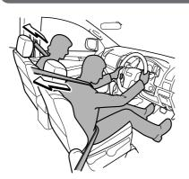
When the vehicle receives an impact exceeding a certain level during a frontal collision, or lateral collision (in models with side airbag and curtain airbag), the fastened seat belt is retracted instantly and removes the slack in the seat belt to securely restrain the driver and the passenger in the seat, thus enhancing the seat belt's restraining effect.
