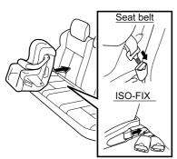
4. Attach the tether hook to the top tether anchorage.
