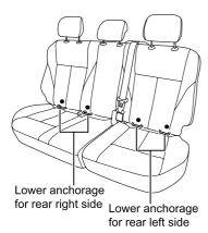
CRS lower anchorages are installed to the outboard seating positions.
