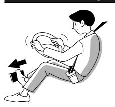
As the brake booster will no longer operate, brake effectiveness will be reduced. The power steering system will not work so the steering wheel will be hard to turn. Stay calm and decrease vehicle speed by pressing the brake pedal. Then, promptly pull the vehicle over to a safe location and inspect its condition. If the engine does not start, contact the nearest Isuzu Dealer.
