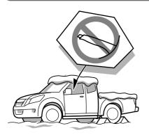
When snow collects around the wheels and lights, try to remove it before night falls. Do not apply the parking brake in cold regions. If you leave the parking brake applied, the wires and brake shoes could freeze up, making it impossible for you to release the parking brake. Be sure to park the vehicle in gear.
