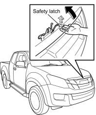
Insert a hand into the space at the front edge of the engine hood, push the safety latch upward and release the lock to open the engine hood.
