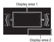
The following is shown on the MID depending on the conditions. If the driving support system information display is selected while the LDW is active, information is displayed in display area 1. On the other hand, if anything other than the driving support system information display is selected, information is displayed in display area 2.
