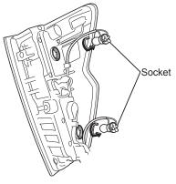
2. Turn the socket of the replacing bulb counterclockwise to remove it.
