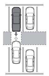
When the detection area of the sensors is blocked by adjacent walls, parked vehicles, etc.
