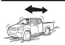
If the vehicle gets stuck in mud, depressing the accelerator pedal more than necessary will simply dig the vehicle deeper into the mud and make it harder to extricate. Either put stones, tree branches or blankets under the tires to gain traction or repeatedly drive forward and backward to use the vehicle's momentum to extricate it.
