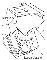
2. Insert latch plate A into buckle A until a clicking sound is heard.
