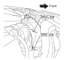
When the engine coolant level in the reserve tank is below the "MIN" line, open the tank cap and fill to near the "MAX" line with engine coolant. Tighten the cap securely after the engine coolant has been replenished.
