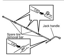
1. Assemble the spare tire removal bars and jack handle.
