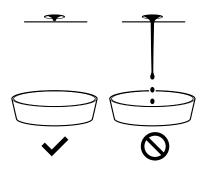
5. Wait until the flow of oil stops and the oil pools into a drop inside the oil pan drain hole.
