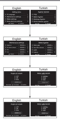
34. Set the maintenance reminder again. Select "Maintenance settings" displayed on the MID screen. Then select "Engine oil". After selecting "ON", adjust the distance as desired by pressing the MID mode R switch or MID mode L switch. Then press the MID mode confirm switch to confirm. When an item is confirmed or "END" is selected, the previous display returns.
