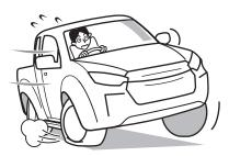
When the tire gets flat while driving, avoid hard braking, hold on to the steering wheel firmly and stop the vehicle.
