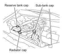
The reserve tank is located at the front right side of the engine compartment. When the engine has cooled down, make sure that the intercooler coolant level in the reserve tank is between the "MAX" and "MIN" line. In addition, check that the intercooler coolant is full to the filler neck of the subtank. Check the intercooler coolant level only when it is cold.
