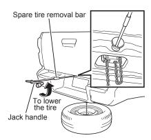
Insert the spare tire removal bar into the hole in the spare tire carrier, and turn the jack handle counterclockwise.
