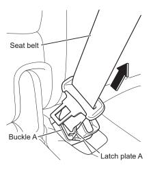
Pull the seat belt in the direction of the arrow and check that latch plate A and buckle A are securely fixed.
