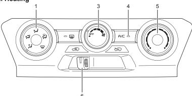
Set the outlet selector dial (1) to the """ or """ position. Use the """ position for warming your feet while defogging the windshield. Set the air selector lever (6) to the """ position.
