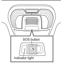
You can check the eCall system status by the lighting status of the indicator light and the buzzer sounds.
