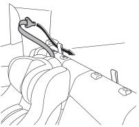
3. Pass the top tether belt from the outboard side through the anchorage toward the inboard side.
