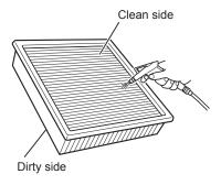
Blow compressed air at a pressure of up to 690 kPa (7.0 kgf/cm²/100 psi) against the clean side of the element to remove the dust.
