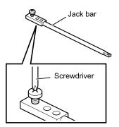
When assemble jack bars to each other, tighten joint bolt by hand or a screwdriver (Phillips side).
