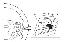
When the adaptive cruise control is set, press the LKAS switch to set the LKAS to
