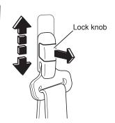
To adjust the anchor height, move the shoulder anchor up or down with the lock knob pulled toward you.
