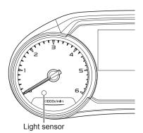
When the power mode is "ON" (models with passive entry and start system) or the starter switch is in the "ON" position (models without passive entry and start system), the illumination brightness is automatically adjusted according to the brightness inside the vehicle. The initial setting is "Automatic". By changing to "Manual", the illumination brightness of both the meter and MID can be individually set.
