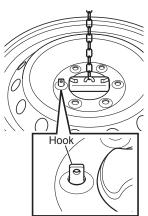
Insert the hook of the plate into the disc wheel nut hole and adjust its position for secure engagement with the spare tire before winding the chain up.
