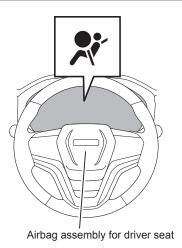
The SRS airbag warning light checks and alerts the conditions of the SRS airbag system.
