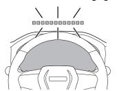
The forward collision warning (FCW) light is a warning light that flashes just before the automatic brake is activated to alert the driver to a risk of a collision with a pedestrian, bicycle rider, vehicle, or obstacle in the forward direction.
