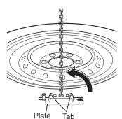
4. Place your fingers through the center of the disc wheel and hold the tabs on the spare tire carrier plate.
