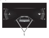
The following is shown on the MID depending on the conditions. If the driving support system information display is selected while the LKAS is active, information is displayed in display area 1. On the other hand, if anything other than the driving support system information display is selected, information is displayed in display area 2.
