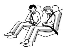
The seat belt with pretensioner and the supplemental restraint system (SRS) airbag system operate when the vehicle is subjected to an impact exceeding a certain level when a collision occurs.
