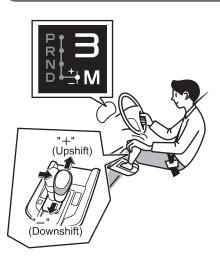
When the selector lever is shifted from the "D" position to the right, the transmission is switched from auto mode to manual mode. In manual mode, the gears can be selected by operating the selector lever to "+" (upshift) or "-" (downshift).
