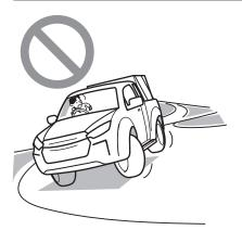
When making a U-turn on a sharp slope, the vehicle is in danger of turning over the moment it crosses the slope. Drive carefully selecting the road surfaces so that the tires on the higher side of the slope may not run on any convex part of the slope surface.
