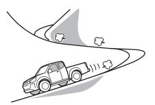
When driving down a long slope, use engine brake together with the foot brakes. Using the low-gear engine brake reduces the work load on the foot brakes and yields greater braking force. In automatic transmission models, do not use the auto mode, as it does not provide engine efficiency. Use only the manual mode for engine braking.
