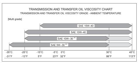
\*1: Use is possible at ambient temperatures of up to 45°C (113°F) in the case of Isuzu genuine oils of grade xxW-30.
