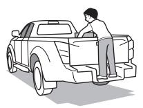
Use the rear step bumper for easy loading and unloading of cargo.
