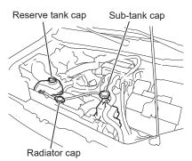
When the intercooler coolant level in the reserve tank is below the "MIN" line, open the tank cap and fill to near the "MAX" line with intercooler coolant. Tighten the cap securely after the intercooler coolant has been replenished.
