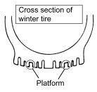
Use winter tires of the same sizes as the standard tires. Also, use wheels of the same size as those with the standard tires. A winter tire has reached its wear limit when the tread grooves have worn to half of the depth of the new tire. At this time, platforms indicating that the tire can no longer give adequate performance on snow become visible in the grooves. Replace the tire with a new one.
