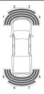
The detection status is displayed on the MID. When the sensors detect an obstacle, the display that indicates the distance between the vehicle and the obstacle comes on red. The distance to the obstacle is indicated separately for each sensor.
