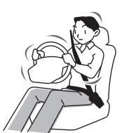
Grasp the steering wheel with both hands, and move it in the axial direction and also up and down, and left and right to see if there is any looseness.
