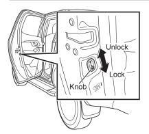
If you place the knob in the lock position and close the door, it will be impossible to open the rear door from inside the vehicle.
