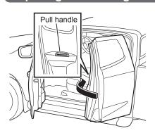
To open the door, push the inside door handle while the front door is open.
