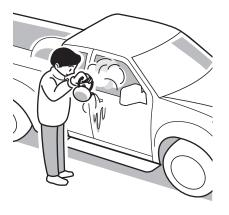
If you try to force the key into the door, you could bend it. And if you try to pull the door open with undue force, the rubber seal around the door could come unstuck or become damaged. Use warm water to melt the ice, then quickly wipe it away and open the door.
