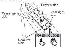
Operate the switch to open or close the window.
