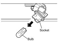
4. Pull out the bulb from the socket.
