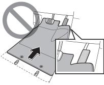
Make sure that floor mats designated for the vehicle model and model year are securely fastened on top of the floor carpet before use. When securing, make sure the clips included with the floor mats are properly installed.
