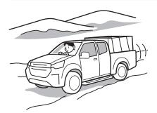
On a snow-covered or icy road, drive at a constant speed and keep your speed low enough to stay completely in control. When applying the brakes, depress the pedal gently several times instead of depressing it strongly. It is dangerous to depress the pedal strongly at once because it could cause the vehicle to slip, making the steering wheel useless.
