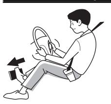
As the brake booster will no longer operate, brake effectiveness will be reduced. The power steering system will not work so the steering wheel will be hard to turn. Stay calm and decrease vehicle speed by depressing the brake pedal. Then, promptly pull the vehicle over to a safe location and inspect its condition. If the engine does not start, contact the nearest Isuzu Dealer.
