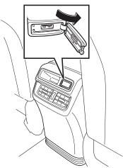
The USB power outlet can be used when the power mode is "ACC" or "ON" (models with passive entry and start system) or the starter switch is in the "ACC" or "ON" position (models without passive entry and start system).
