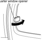
The quarter window on each side can be opened and closed by operating the quarter window opener.
