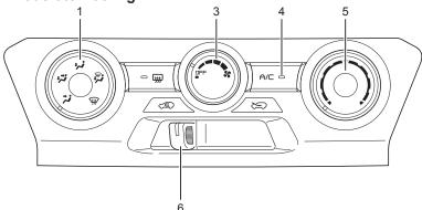
This setting is suitable for extended periods of cooling or moderate cooling. Press the A/C switch (4) to turn it on.
