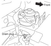
The fuel filter is located at the rear left side of the engine compartment.
