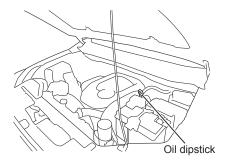
Perform the engine oil level check on a flat surface while the engine is cold before starting it. If the engine has already been started, stop it after it has sufficiently warmed and wait 30 minutes or more before performing.
