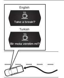
When the system detects that the vehicle is weaving while the vehicle is driving at approximately 60 km/h (37 MPH) or more, a warning is issued. A warning message is displayed on the MID. At the same time, a buzzer sounds.
