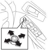
2. Operate the switch to adjust the angle of the mirror.
