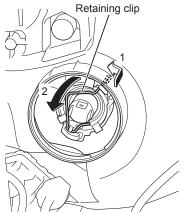
3. Disconnect the connector from the bulb. Remove the connector by pushing the tabs.
