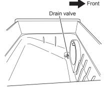
4. Clean the drain valve at the bottom of the air cleaner.
