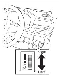
This switch is used to adjust the brightness of the illumination in the instrument panel. Turning the switch up brightens the lights, and turning the switch down darkens them. The brightness can be adjusted with the light control switch in the "AUTO" (with the taillights "ON"), "-00-" or "
