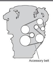
The tension of the accessory belt is automatically adjusted using an autotensioner.
