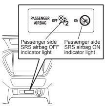
Passenger side SRS airbag ON indicator light
