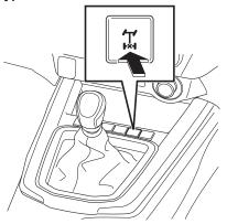
To engage the differential lock, press the rear differential lock switch.
