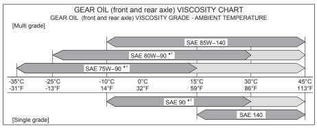
\*1: Use is possible at ambient temperatures of up to 45°C (113°F) in the case of Isuzu genuine oils or other recommended oils of grade xxW-90.
