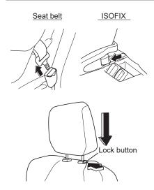
3. Unfasten the seat belt or the ISOFIX anchorages to remove the CRS.
