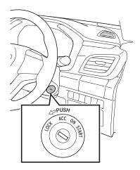
LOCK : In this position, the key can be inserted or removed.
