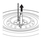
Stand the spare tire carrier plate so that it is perpendicular to the disc wheel, and remove the spare tire carrier plate through the center of the disc wheel.
