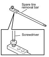
When assembling the spare tire removal bars to each other, tighten the joint bolts by hand or with a screwdriver (Phillips head).
