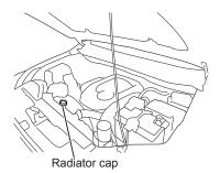
The reserve tank is located at the front right side of the engine compartment. When the engine has cooled down, make sure that the engine coolant level in the reserve tank is between the "MAX" and "MIN" line. In addition, remove the radiator cap and check that the engine coolant is full to the filler neck. Check the engine coolant level only when it is cold.
