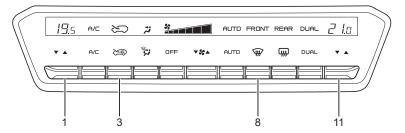
Operate the windshield defroster switch (8) and turn on the defroster. The display will show the "FRONT" symbol. The air conditioning system starts operating.
