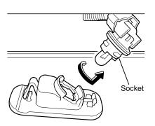
3. Loosen the socket by turning it counterclockwise.
