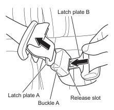
2. Insert latch plate B into the release slot of buckle A.
