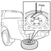
1. Set the disc wheel so that its outer surface faces up, and then insert the plate into the center of the disc wheel.
