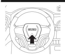
To sound the horn, press the pad with a horn symbol on the steering wheel.
