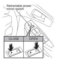
The retractable power mirror switch is active only when the power mode is "ACC" or "ON" (models with passive entry and start system) or the starter switch is in the "ACC" or "ON" position (models without passive entry and start system).
