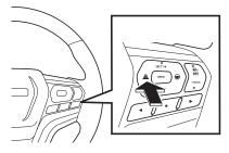
Press the main switch to turn on the adaptive cruise control. The adaptive cruise control indicator light comes on white.
