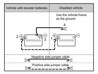
4. After connecting the cables, start the engine of the vehicle with the booster battery. Slightly rev up the engine of the vehicle with the booster battery and start the engine of the disabled vehicle.
