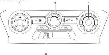
Turn the outlet selector dial (1) to the preferred position. Move the air selector lever (6) to the "" position. Set the temperature control dial (5) to the preferred position depending on the season and climate.
