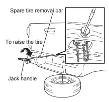
Let the chain rest in the center of the disc wheel while it is raised halfway. Then turn the jack handle to lift up the tire.
