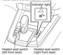
The heated seat can be used when the power mode is "ON" (models with passive entry and start system) or the starter switch is in the "ON" position (models without passive entry and start system). Every time the switch is pressed, it switches between high, low, and off.
