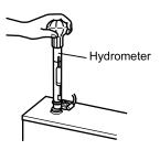
Check the specific gravity of the battery fluid using a hydrometer. If the specific gravity is too low, the battery should be charged.
