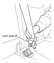
Pull out the seat belt so that latch plate B faces the vehicle center. Do not let the seat belt twist as you pull it out.
