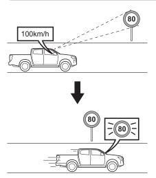
When your vehicle speed exceeds the speed of the maximum speed sign detected by the stereo camera, the maximum speed sign displayed on the MID flashes.
