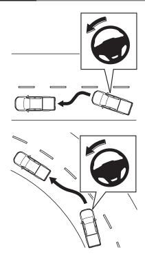
The system recognizes lanes and assists the steering wheel operations to keep the vehicle driving in the center area of the lane while driving at a speed of approximately 60 to 130 km/h (37 to 80 MPH) while the adaptive cruise control is set.
