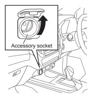
You can use this when the power mode is "ACC" or "ON" (models with passive entry and start system) or the starter switch is in the "ACC" or "ON" position (models without passive entry and start system).
