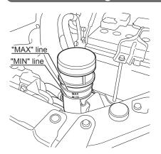
The reserve tank is located at the front of the engine compartment on the left. The fluid level is correct if it is between the "MAX" and "MIN" lines on the reserve tank. If the level is lower than the "MIN" line, add power steering fluid up to the "MAX" line. Furthermore, perform an inspection for power steering fluid leaks.
