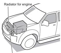
Radiator for water-cooled intercooler
