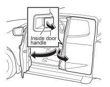
To open the door, after first opening the front door, pull the inside door handle and open the side access panel.
