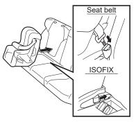
Attach the CRS by using the seat belt or the ISOFIX anchorages. Refer to the instruction manual of the CRS.
