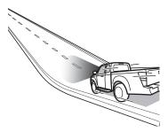
Under the following road conditions or conditions of your vehicle, the stereo camera may not be able to detect the preceding vehicle. Vehicles in neighboring traffic lanes or roadside objects may also be incorrectly detected. Under conditions such as these, do not use the adaptive cruise control. If cruise control is currently in use, operate the brake pedal and take other actions as necessary.
