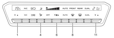
Operate the windshield defroster switch (8) to turn on the defroster. The display will show the "FRONT" symbol. The air conditioning system starts operating. The defroster is automatically set to the outside air ventilation mode.
