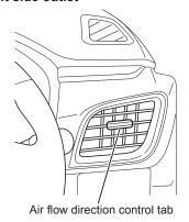
To close the front side outlet, move the tab outward.
